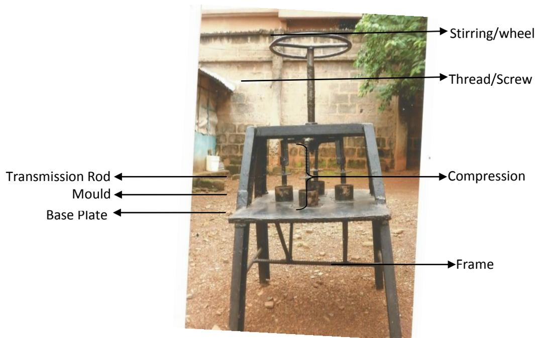
Plate 1.0: The fabricated screw press.
